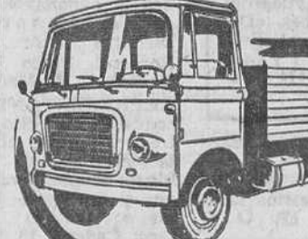
TIPOS SH-400 SH-550 MOTOR BMC 77 HP CAJA + CARGA 4.250 Kgs. 5.800 Kgs.
