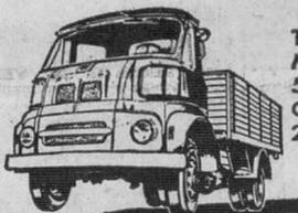
TIPOS S-66, MOTOR BMC. 56 HP, CAJA + CARGA 2.500 KGS
