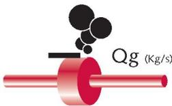
$$Q_g = \varphi \cdot c \cdot A \cdot \left[ \gamma \left( \frac{2}{\gamma + 1} \right)^n \right]^{0,5} \cdot \frac{P}{\left( \frac{R \cdot T}{M} \right)^{0,5}}$$
