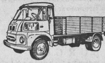
TIPOS: MOTOR BMC CAJA + CARGA 5-66 5-78 56-HP 77-HP 2.500 Kgs. 4.100 Kgs.
